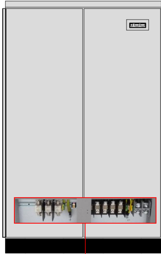
TPS/T/D 90KVA REAR PANEL
