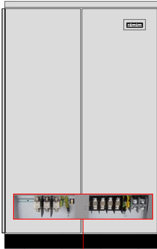
TPS/T/D 90KVA PANNELLO POSTERIORE
